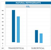
Testing conditions data reference: Transcritical: Evap. T. -10°C; Gas cooler out T. 33°C; Gas cooler pressure 83,7 bar, Superheating 10K; Subcritical: Evap T. -30°C, Cond. T. +10°C; Superheating 10K;
