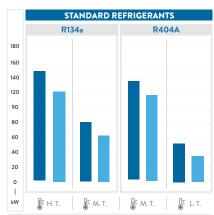
Testing conditions data reference: H.T.: evap. T. +5°C; cond. T. +50°C M.T.: evap. T. -10°C; cond. T. +45°C L.T.: evap. T. -35°C; cond. T. +40°C
